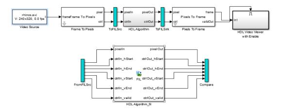
The blue ToFILSrc bar branches the pixel-stream input of the HDL Algorithm block to the FromFILSrc bar on the input of the HDL Algorithm\_fil block. The second blue bar branches the pixel-stream output of the HDL Algorithm block into the Compare subsystem, where it is compared with the output of the HDL Algorithm\_fil block. For image and video processing, this setup can be slow because it sends only a single pixel, and its associated control signals, in each packet to and from the FPGA board.
